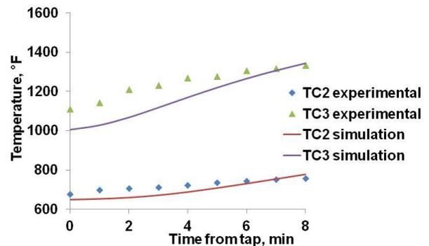
Figure 12. Graph shows the comparison between experimental and CFD simulated lining temperature for 100 lb (45 kg) ladle lined with the novel refractory (silica + 30 vol. % cenospheres).<sup>3</sup>
