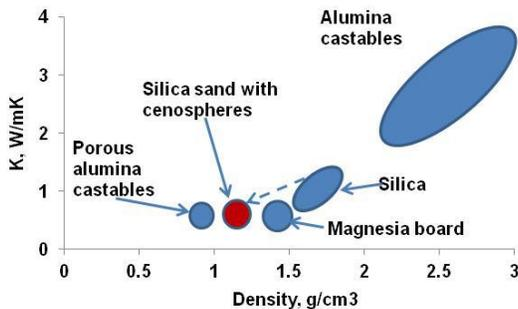
**Figure 1. Room temperature thermal conductivity versus density of different refractory materials<sup>3</sup> is shown. (Artwork courtesy of ST Foundry, Inc.)**
