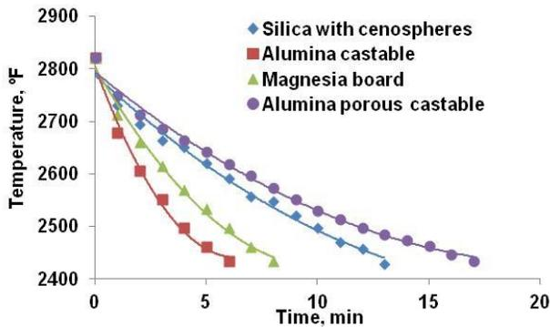
**Figure 13. A graphical comparison of cooling curves for developed and previously studied linings.<sup>3</sup>**
