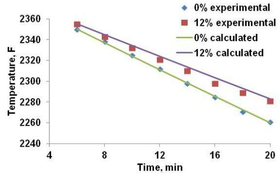
Figure 11. Graph shows the comparison between the experimental and theoretical temperature drop for experimental molds with the silica sand and the novel refractory (silica + 30 vol. % cenospheres).<sup>3</sup>
