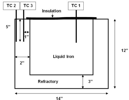
**Figure 6. This is a schematic of the laboratory ladle 100 lb (45 kg) prepared for Experiment 2.<sup>3</sup>**
