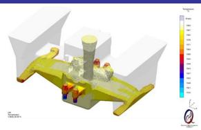
Temperature profile during filling of the test component with molten metal. Filling and solidification were computer simulated prior to actual pouring to assure best properties and absence of internal porosity defects.
