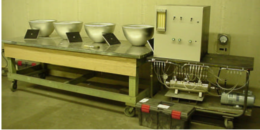
Figure 11 Storage Domes and Sampling Apparatus
