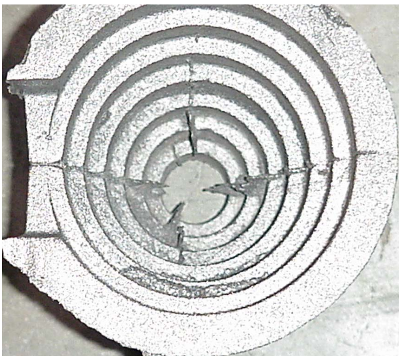
Median Appearing Casting from Mold FR 001 – Baseline
