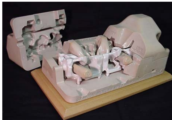
Figure 2.1.2 Typical Mold and Core Package
