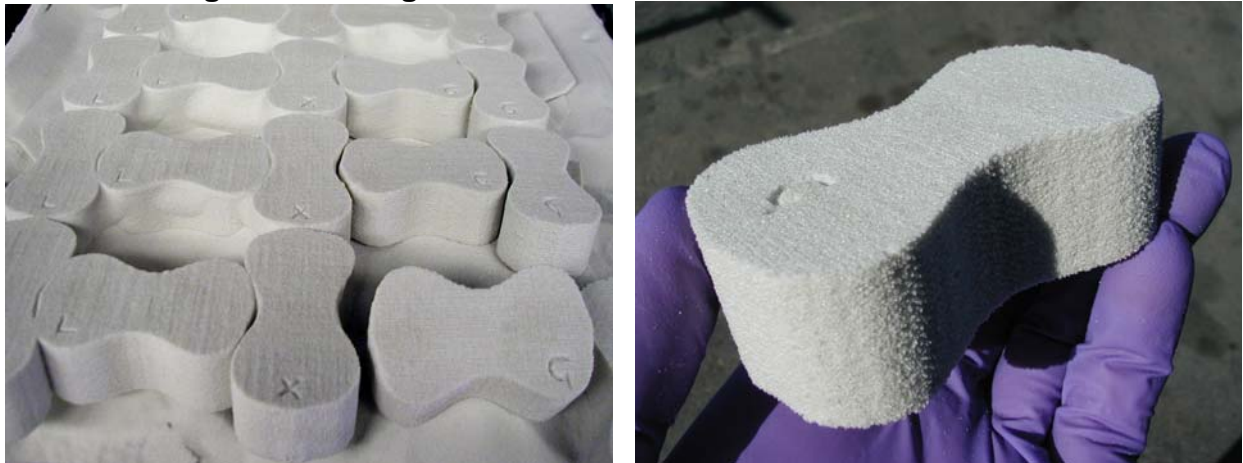
Figure 3.2.1 Dogbone Cores in As-Printed and After Removal
