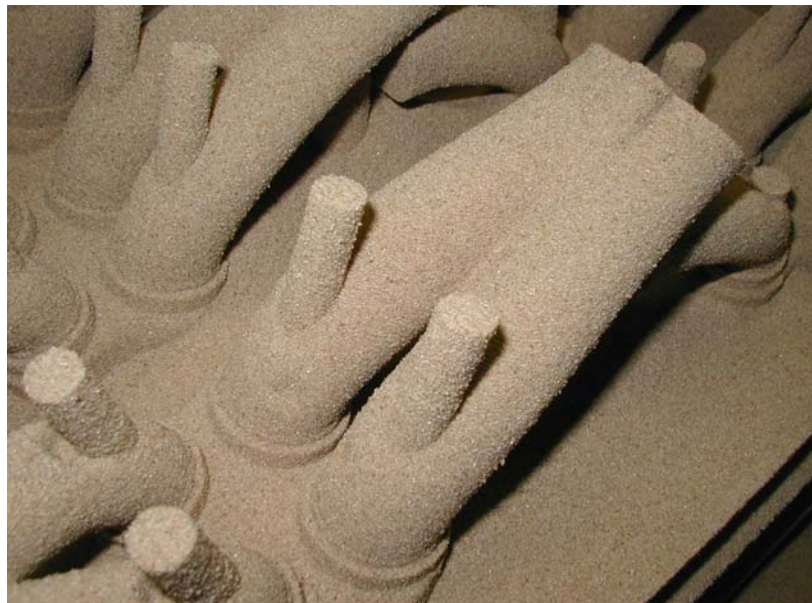
Figure 3.2.3 Cylinder Head Port Cores in Print Box Done with Lakesand
