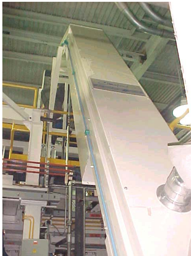
Figure 2-4 Enclosed Belt Conveyor
