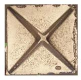
Figure 7 Edge Deformation Caused by Gas Bubbles
