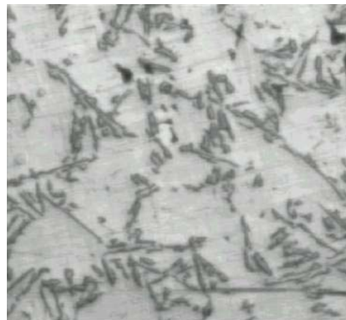
b) Conventional - coarse eutectic structure.
