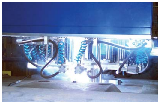
c) Close view of plasma arc system while energized.
