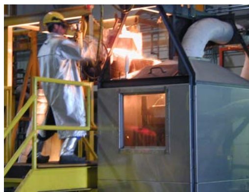
Figure 2-3 Metal Pouring into Test Casting Molds
