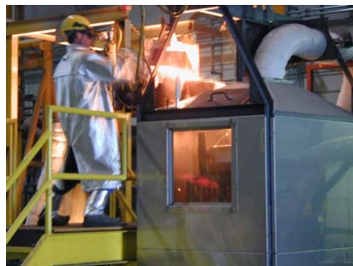
Figure 2-3 Metal Pouring into Test Casting Molds
