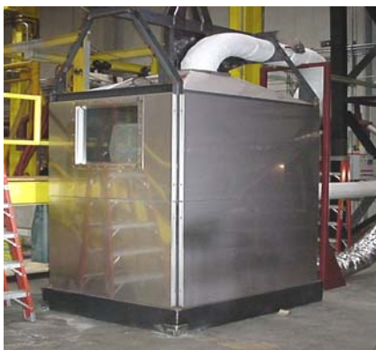
Figure 2-2 Technikon Research Foundry Emission Collection Hood
