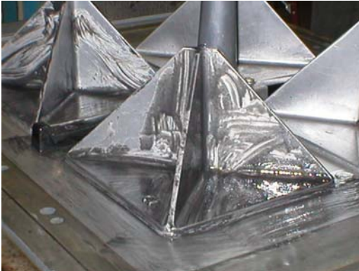
Figure 4 Green Sand Release Agent on Pattern
