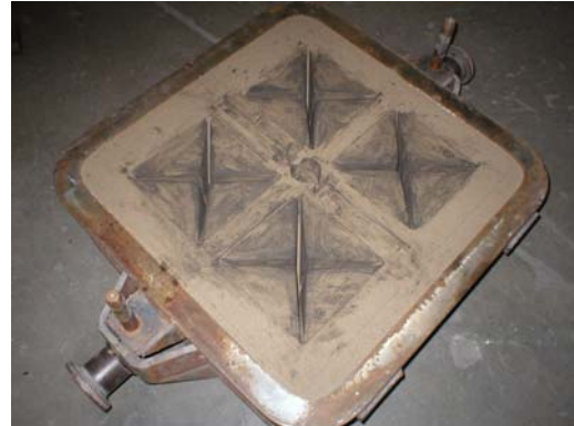
Figure 5 Release Agent (Transferred) on Mold
