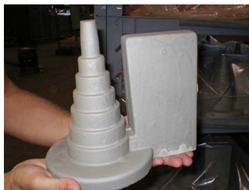
Figure 8 Sample Core containing Additive
