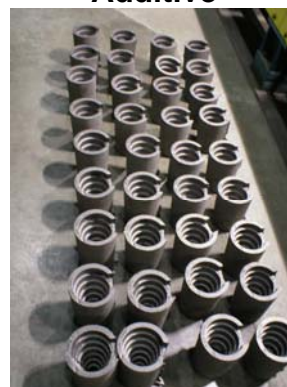
Figure 8 Sample Core containing Additive
