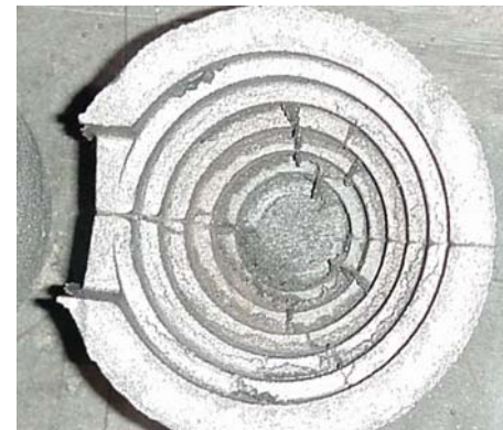
Figure 15 Median Appearing Casting from Mold FR 010 – Black Iron Oxide
