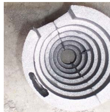
Figure 17 Median Appearing Casting from Mold FT005 – Blender Material
