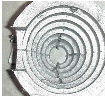
Figure 14 Median Appearing Casting from Mold FR 005 – Red Iron Oxide
