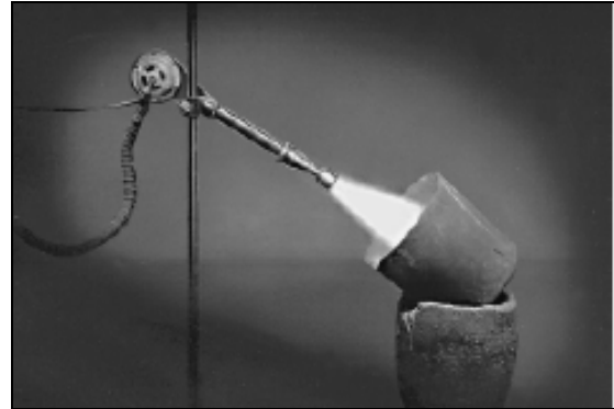
Figure 3-1 Natural Gas Ladle Preheater
