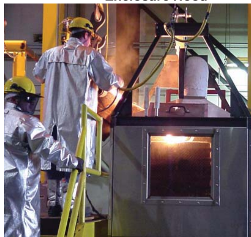
Figure 2-4 Pouring Iron into Mold inside Total Enclosure Hood
