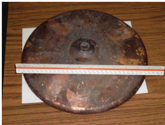
Figure1: MW melted and cast Cu, 30 lbs.
