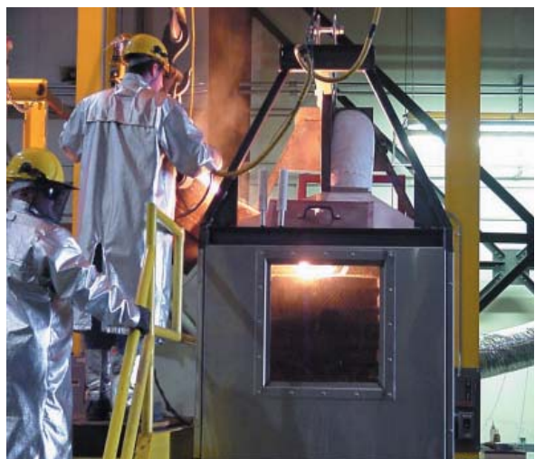
Figure 2-4 Pouring Iron into Mold inside Total Enclosure Hood
