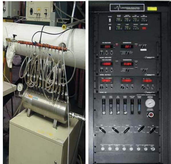
Figure 2-5 Stack Sampling Equipment a) Sampling Train b) E-Bench
