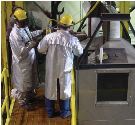
Figure 2-4 Pouring Aluminum into Mold inside Total Enclosure Hood
