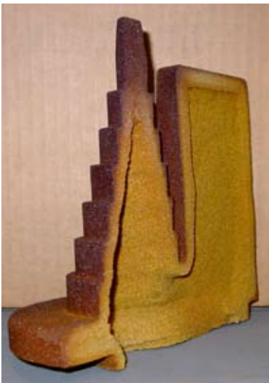
Figure 2-3 Cross Section of Shell Step Core
