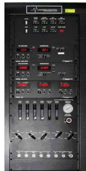
Figure 2-4 Stack Sampling Equipment a) Sampling Train b) E-bench
