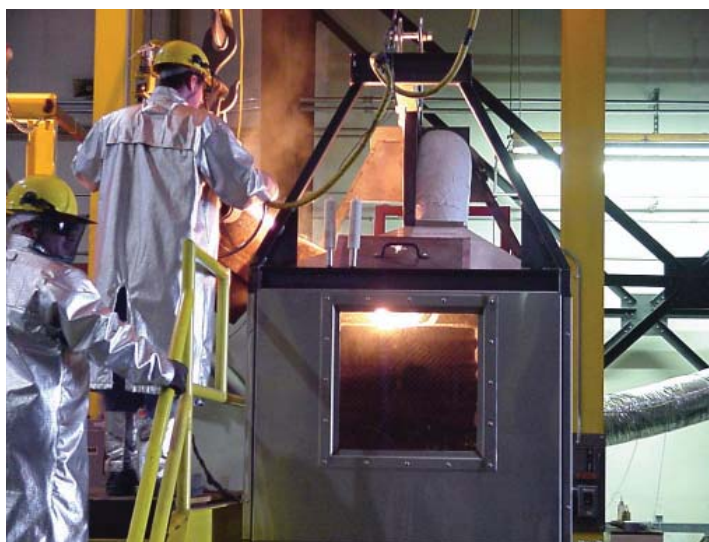
Figure 2-3 Pouring Metal into Mold inside Total Enclosure Hood
