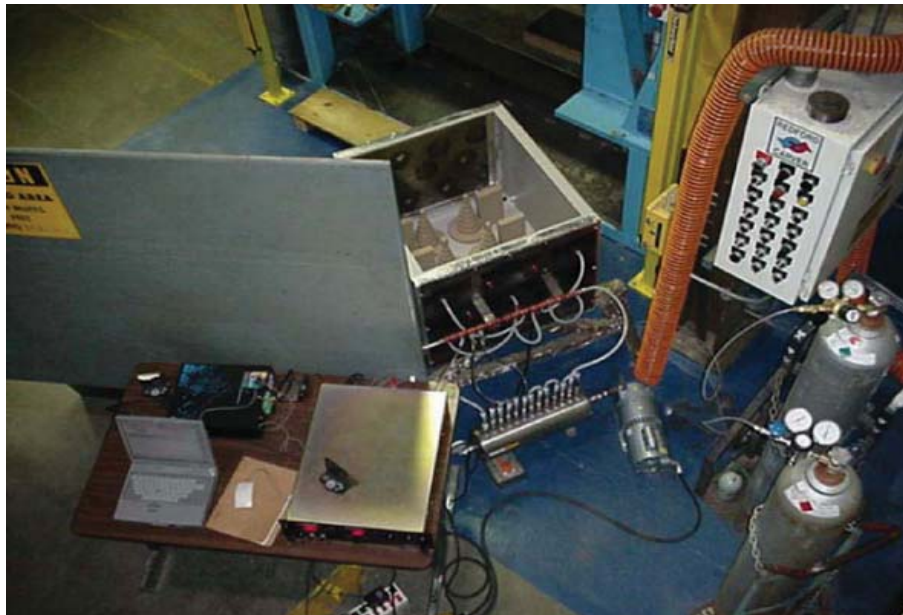
Figure 2-4 Step Core Storage Enclosure and Sampling Train
