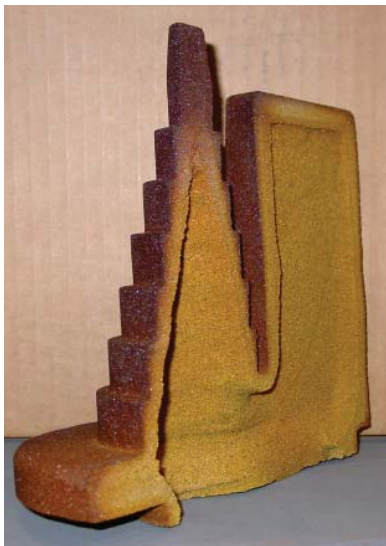
Figure 2-3 Cross Section of Shell Step Core
