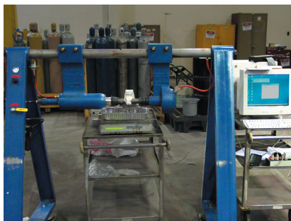
Figure 2-7 Herschal Hammer Shakeout Setup
