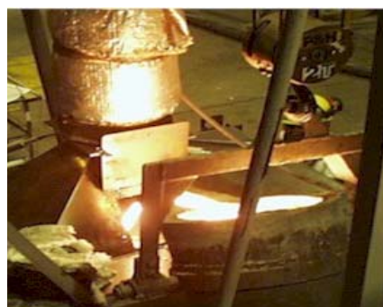
Pouring of Molds Through Opening in Collection Hood
