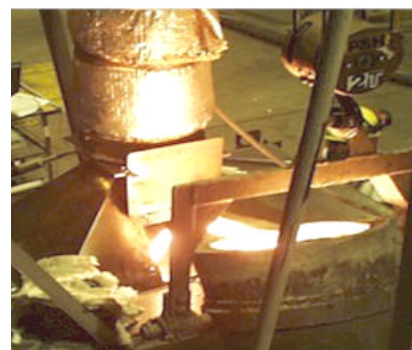
Pouring of Molds Through Opening in Collection Hood
