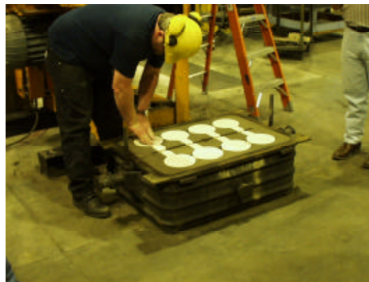
Setting of Step Cores in Mold
