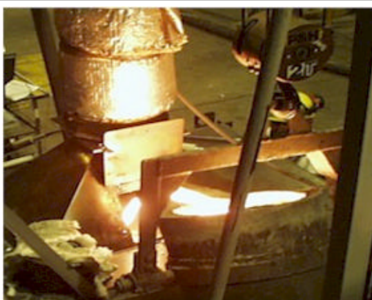
Pouring of Step Core Molds Through Opening in Collection Hood
