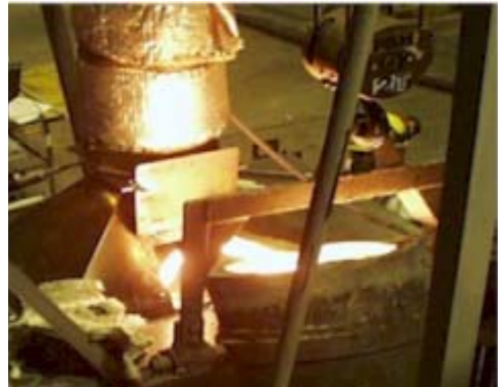
Pouring of Step Core Molds Through Opening in Collection Hood
