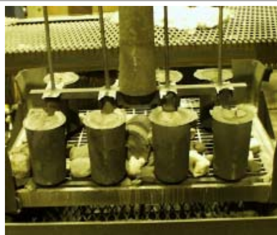
Castings on the Shake Out Deck
