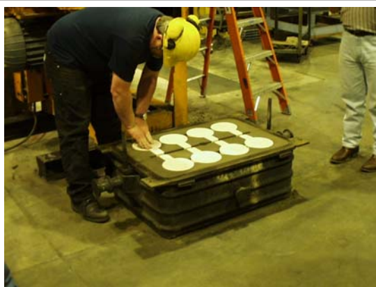
Setting of Step Cores in Mold
