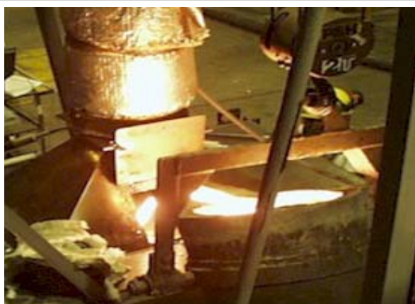
Pouring of Step Core Molds Through Opening in Collection Hood
