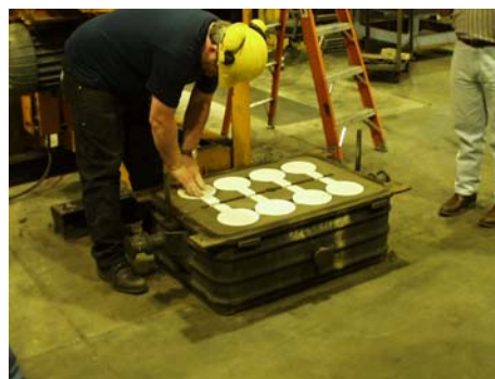
Setting of Step Cores in Mold
