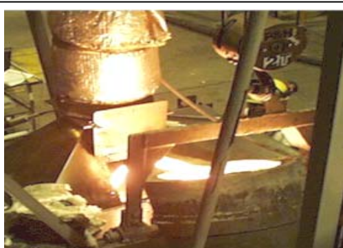
Pouring of Molds Through Opening in Collection Hood
