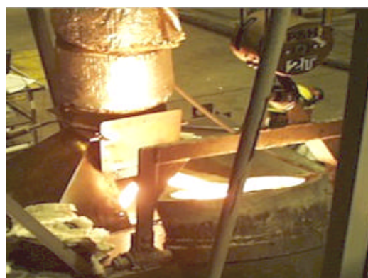
Pouring of Molds Through Opening in Collection Hood
