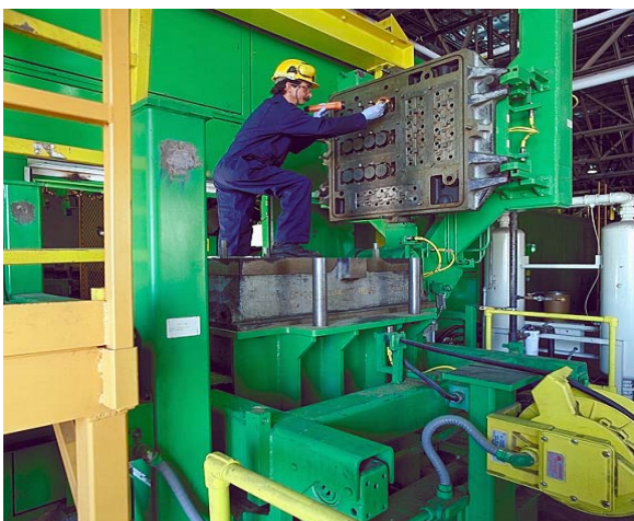
GF Core Machine and Headslab & Water jacket tooling
