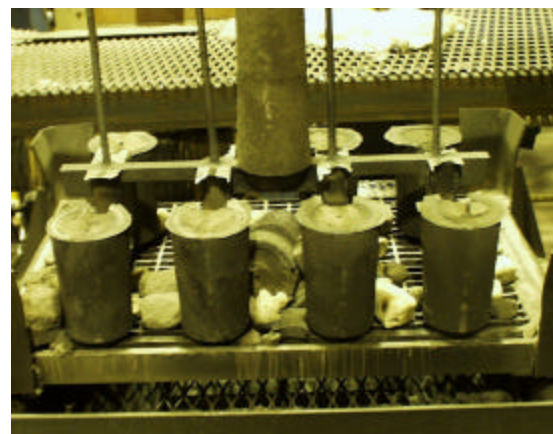
Castings on the Shakeout Deck
