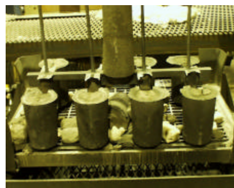
Castings on the Shakeout Deck
