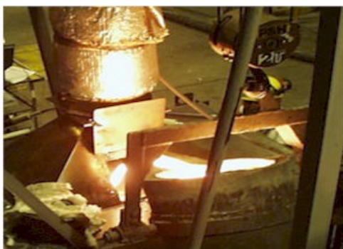
Pouring Step Core Molds Through Opening in Collection Hood
