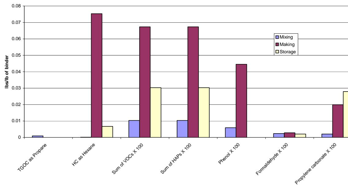
**Figure 3-2. Test ET Average Emissions Results – 1.75% Binder – Lb/Lb Binder**
