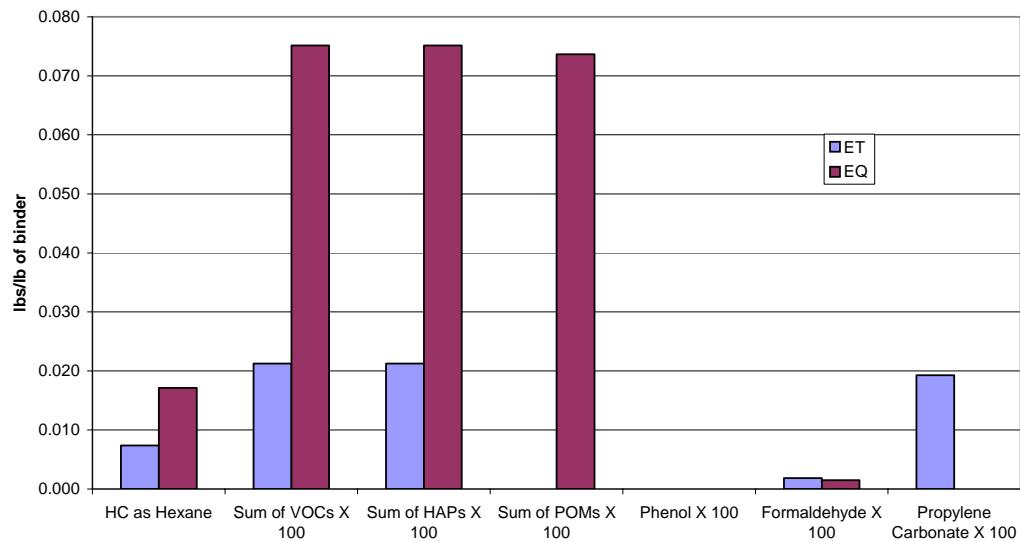
**Figure 3-6. Tests ET Average Emissions Results – 1.20% Binder – Lb/Tn Sand**
