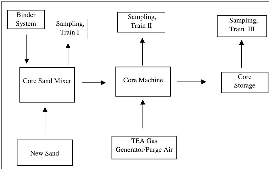
**Figure 2-1. Core Making and Testing Process**
