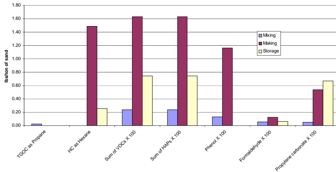
**Figure 3-8. Tests EQ and ET Core Mixing Comparison – 1.75% Binder – Lb/Tn Sand**
