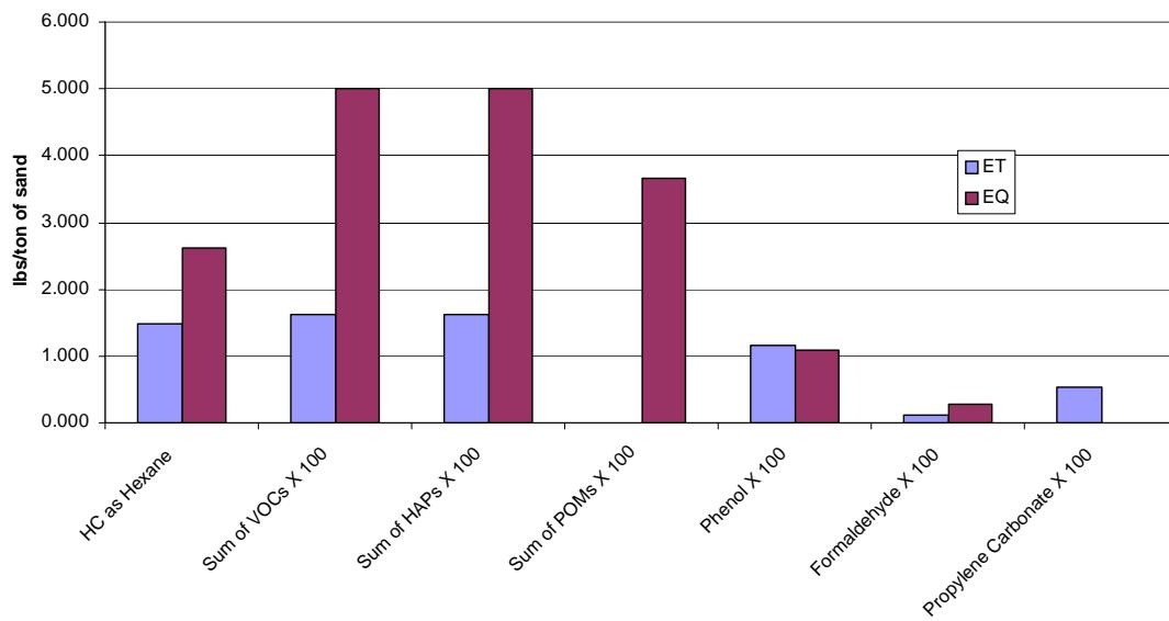
**Figure 3-10. Tests EQ and ET Core Storage Comparison – 1.75% Binder – Lb/Tn Sand**
