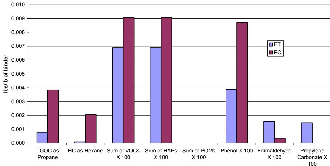
**Figure 3-4. Tests EQ and ET Core Making Comparison – 1.75% Binder - Lb/Lb Binder**
