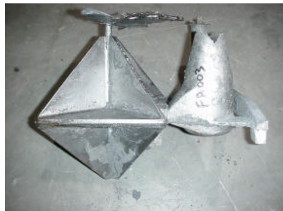
Figure 2-2a Thin walled Star Casting with Gating Attached.
