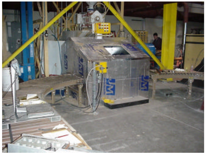
No-Bake Mold Line with Total Enclosure
