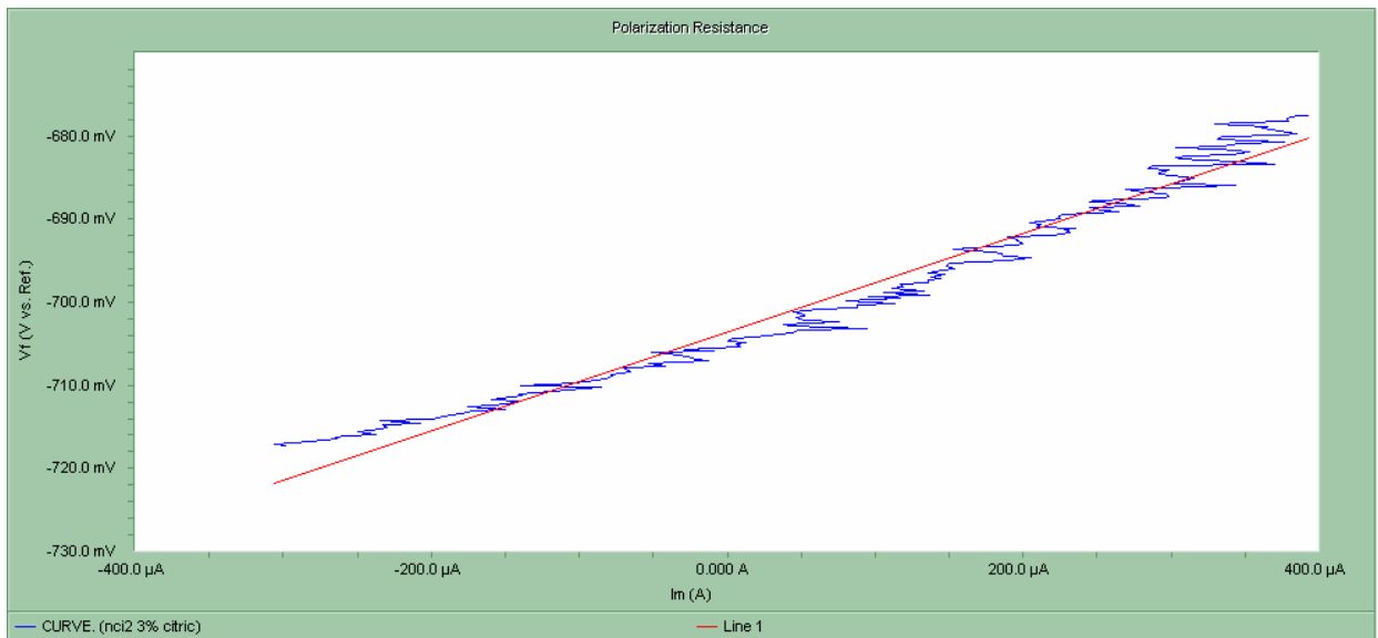
Figure 9: Nodular Cast Iron Sample 2 - Corrosion Rate: 24.43 mpy
