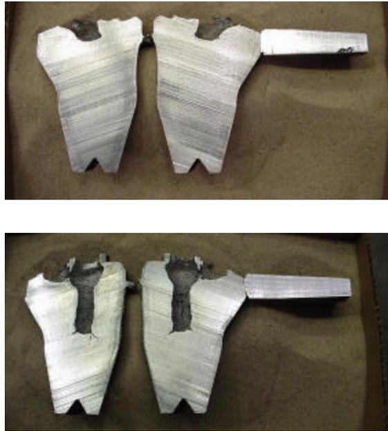
**Figure 3-13 Thermal Profile of the Center of Castings -FG006P and FG006S**
