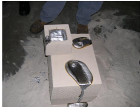
Mold after being poured and stimulated. Shows stimulation hole in rear where stimulator was and flow off vent in front. Aluminum was poured in box and drained to level of top of mold
