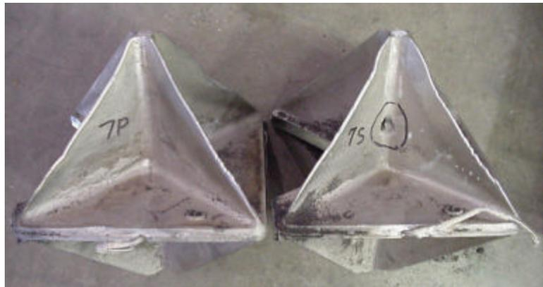
**Figure 3-16 Risers and Gating Connections to Castings - FG007P and FG007S**
