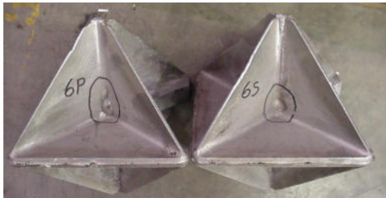
**Figure 3-12 Risers and Gating Connections to Castings FG006P and FG006S**
