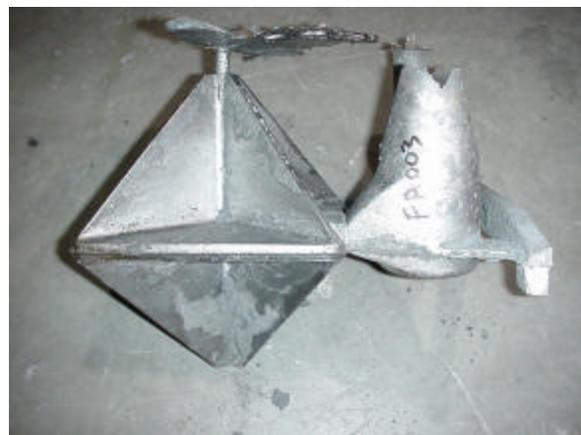
*Variable finned Star Casting with Riser and Gating*
