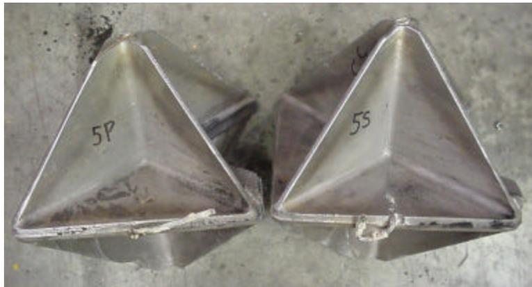
**Figure 3-8 Risers and Gating Connection to Casting for FG005P and FG005S**
