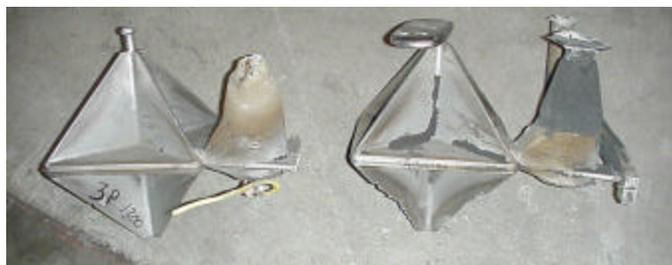
couples failed. The pour temperature was raised 50°F to make the casting less prone to misrun. The extra heat was ineffective indicating that the misrun was due to internal splashing of the initial metal. FG003P had a vented riser. The riser for FG003S was necessarily open to accommodate the stimulator rod. Poured at 1314 Deg F.
