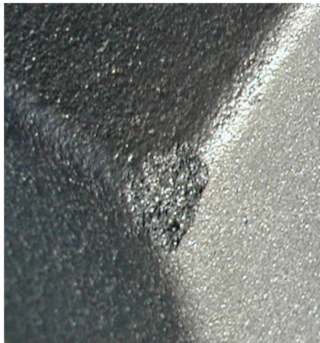
Fusion penetration on surface of gray cast iron near hot spot
