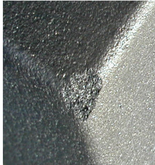
Figure 4-2 Fusion Penetration on Surface of Gray Cast Iron Near Hot Spot
