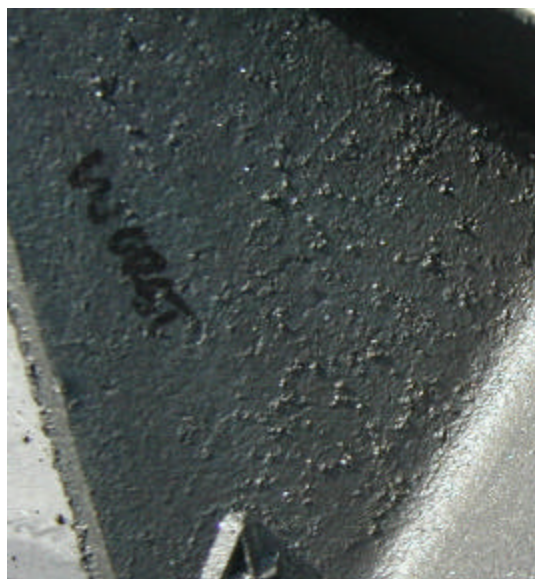
Figure 4-3 Weak Sand Grains Torn Out of the Mold at Mold Stripping (Positive Relief) and Loose Sand aka Dirt (Negative Relief)
