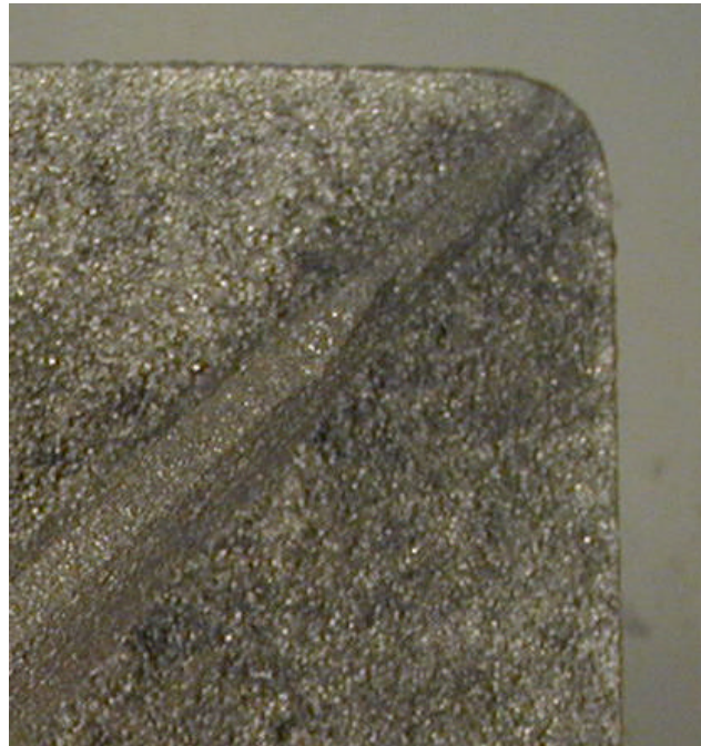
Metal penetration aka burned in sand on flat surface of gray cast iron
