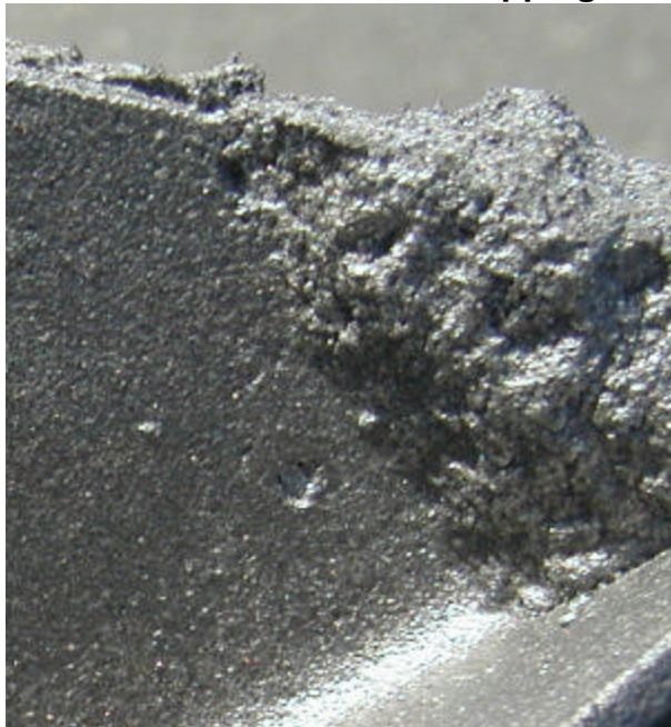
Figure 4-4 Broken Mold Created at Mold Stripping
