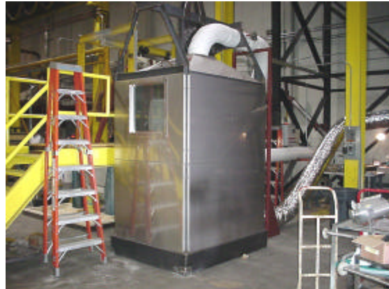
Total Enclosure Test Stand
