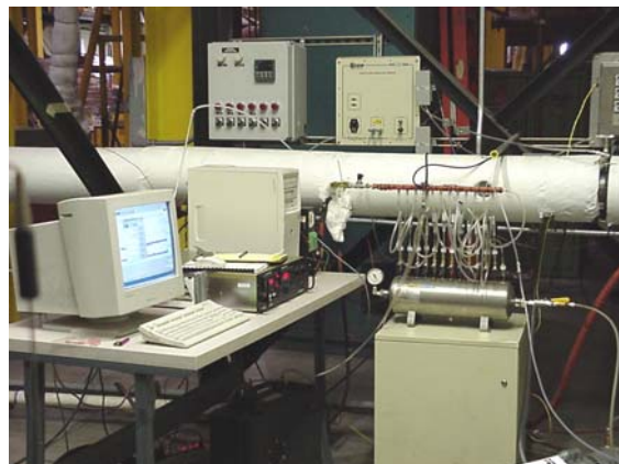
Method 25A (TGOC) and Method 18 Sampling Train
