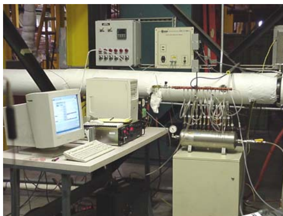
Method 25A (TGOC) and Method 18 Sampling Train
