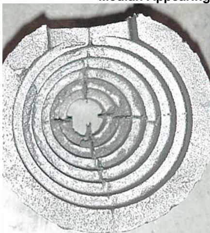
Median Appearing Casting from Mold FR001 & GH006
