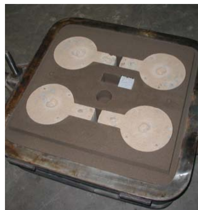
Uncoated Step Cores in mold
