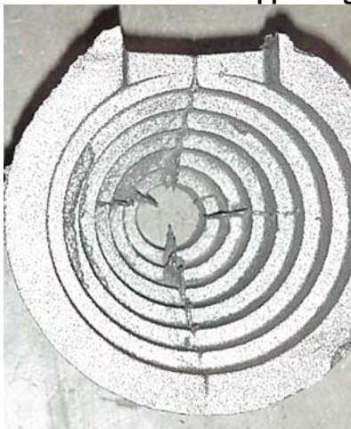
Best Appearing Casting from Mold FR003 & GH008
