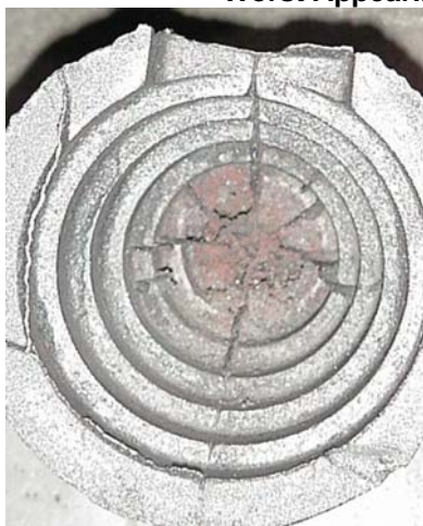
Worst Appearing Casting from Mold FR004 & GH010
