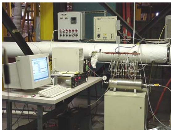
Method 25A (TGOC) and Method 18 Sampling Train
