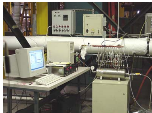
Figure 2-4 Method 25A (TGOC) and Method 18 Sampling Train
