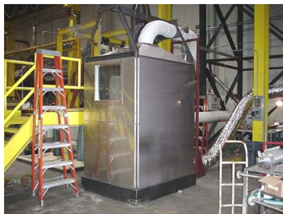
Figure 2-4 Method 25A (TGOC) and Method 18 Sampling Train
