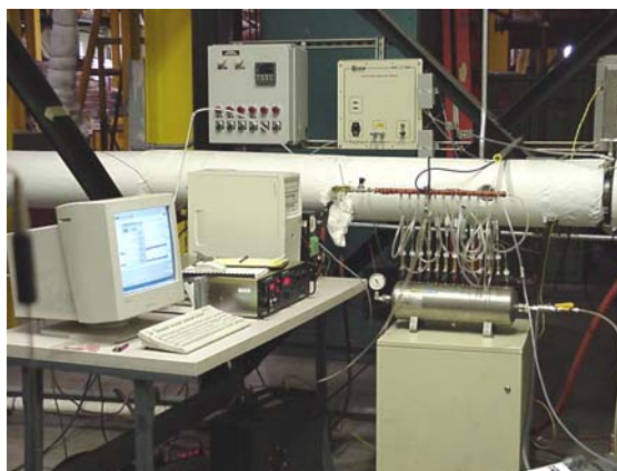
Figure 2-4 Method 25A (TGOC) and Method 18 Sampling Train
