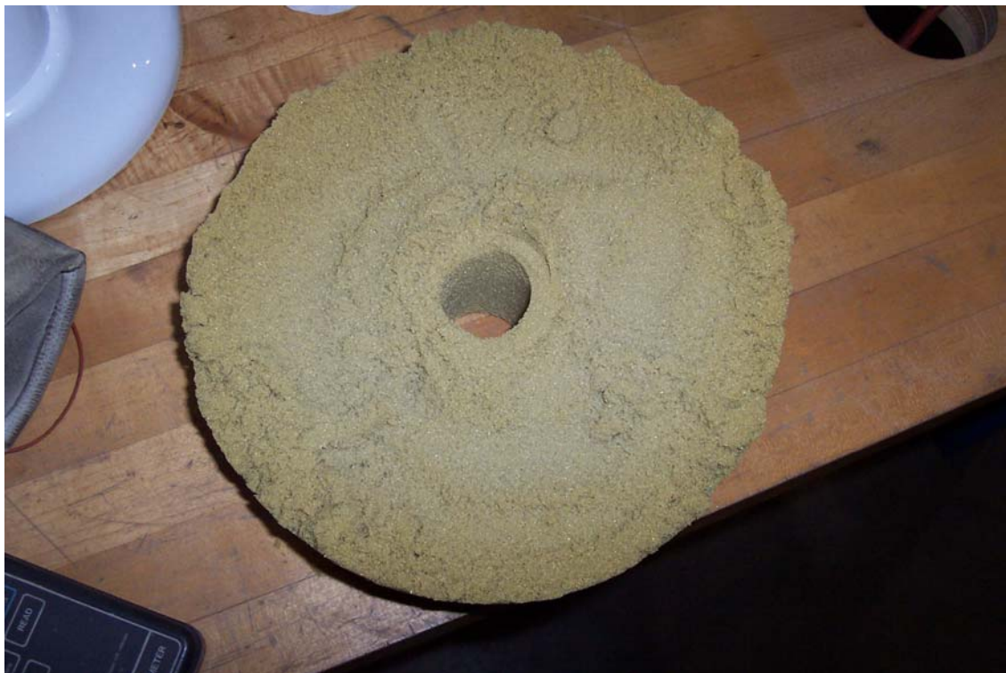
Figure 2-8 Sand/Binder Mixture after completion of test
