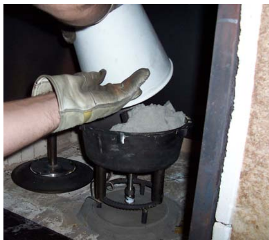
Figure 2-6 Sand/Binder Mixture Evenly Spread in the Holding Chamber
