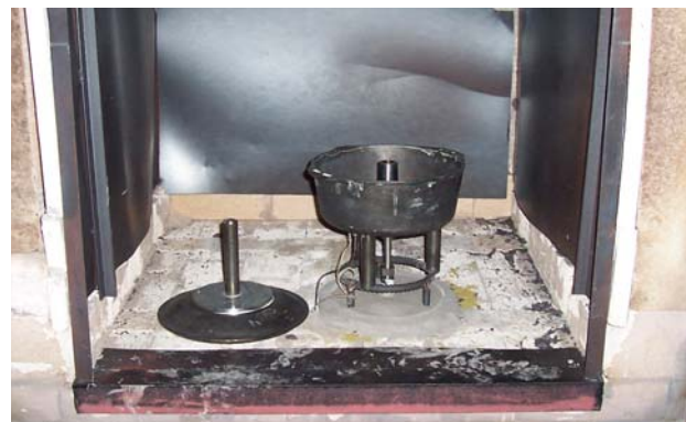
Figure 2-2 Holding Chamber placed in the AccuTherm Oven
