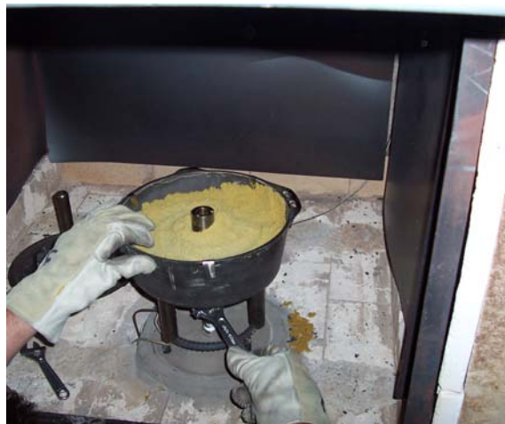
Figure 2-6 Sand/Binder Mixture Evenly Spread in the Holding Chamber
