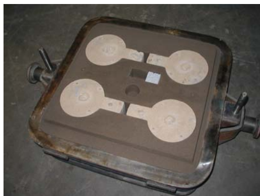
Figure 2-3 Sodium Silicate Cores embedded in a Greensand Mold
