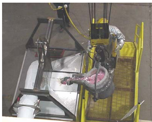
Figure 2-5 Metal pouring from ladle to mold in the TTE
