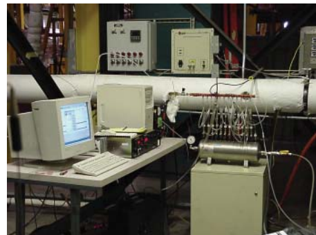
Figure 2-6 Method 25A (TGOC) and Method 18 Sampling Train
