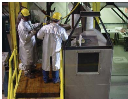
Figure 2-4 Pouring Metal into Mold in Total Enclosure Hood
