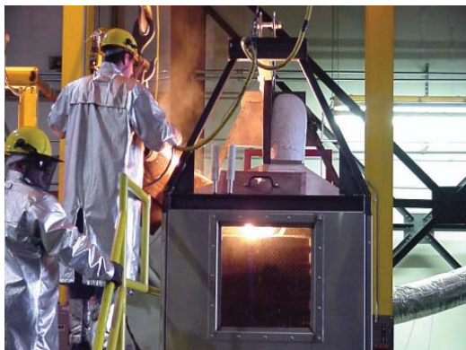
Figure 2-3 Pouring Metal into Mold Inside Total Enclosure Hood
