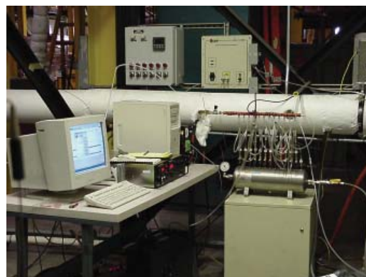
Figure 2-4 Method 25A (TGOC) and Method 18 Sampling Train
