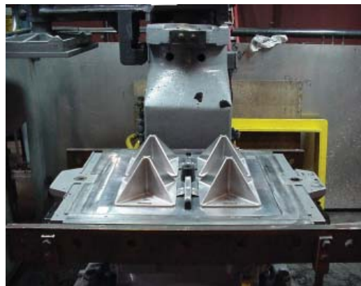
Figure 2-2 Four Cavity Star Pattern
